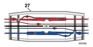
2. Install connection cover (36) over each fluid connection.
