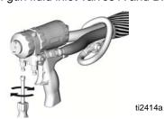
12. Disengage gun piston safety lock.
