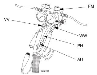
Manifold hose fittings (VV, WW) allow use of 1/4 in. and 3/8 in. ID Reactor heated fluid hoses.
