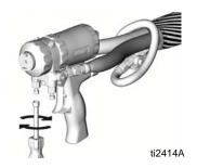
17. Disengage gun piston safety lock.
