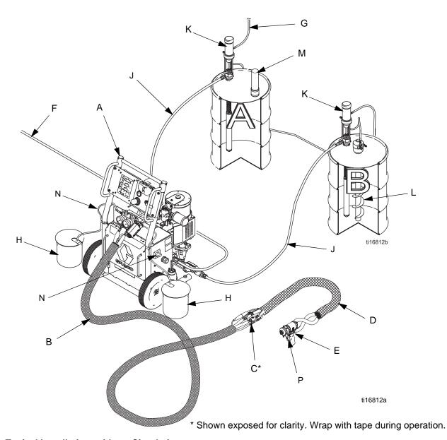
Fig. 1: Typical Installation, without Circulation
