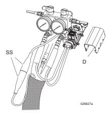
Connect cables (SS). Connect electrical connectors (NN). Be sure cables have slack when hose bends. Wrap cable and electrical connections with electrical tape.
