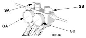
10. Check fluid pressure gauges (GA, GB) to ensure proper pressure balance. If imbalanced, reduce pressure of higher component by slightly turning PRESSURE RELIEF/SPRAY valve for that component toward PRESSURE RELIEF/CIRCULATION, until gauges show balanced pressures.
