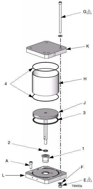
Torque tie rods to 17-22 ft-lbs (1.9-2.5 N•m).
