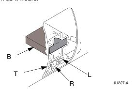
2 309575A 3. Install spring (S) so it will uncoil onto brush (B), as shown. Spring will be damaged if installed backwards.
