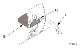
2. Slide terminal (L) under terminal screw (R). Make sure motor lead terminal (T) is still connected at screw. Tighten screw. Be sure brush is free to move down as it wears.
