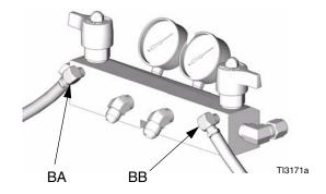
**b.** Alternately: Secure supplied bleed tubes (N) in grounded, sealed waste containers (H). See Fig. 2, page 8.
