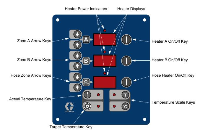
Fig. 4. Temperature Controls and Indicators
