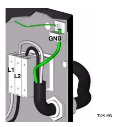
**230V, 3 phase:** Using 5/32 or 4 mm hex allen wrench, connect three power leads to L1, L2, and L3. Connect green to ground (GND).
