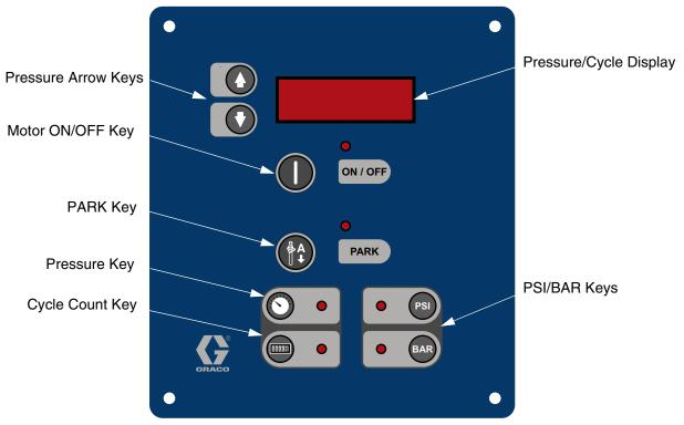
Fig. 5. Motor Controls and Indicators
