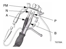
Manifold hose adapters (N, P) allow use of 1/4 in. and 3/8 in. ID fluid hoses. To use 1/2 in. (13 mm) ID fluid hoses, remove adapters from fluid manifold and install as needed to connect whip hose.
