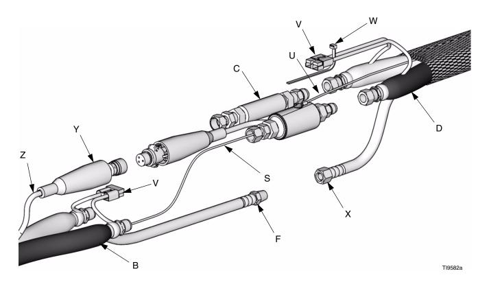
Fig. 6. Install Fluid Temperature Sensor (FTS)
