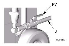
Supply hoses from feed pumps should be 3/4 in. (19 mm) ID.
