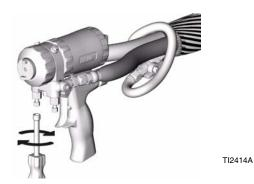
**10.** Disengage gun piston safety lock.
